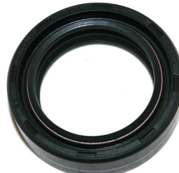
FORK OIL SEAL (GREEN) JAPAN 30*42*11 SPLENDOR / PULSAR / KB4S / VICTOR / STARCITY VFOS005
